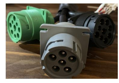
6-Pin – 6to9 adapter Type 1 9-Pin – Black Type 1 – Green Type 2 – Green Type 2 Paccar (check door jam) \*\*Don't forget the 10FT 9-Pin Type 1
