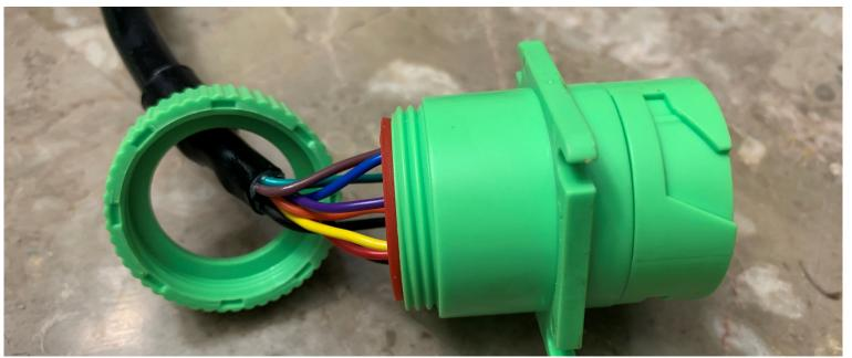
Remove the screw cap at the back of the core connector and slide the cap away.
